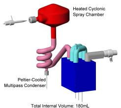
Custom temperature settings for heater and cooler. Patented flow path design ensures rapid wash-in / washout.
